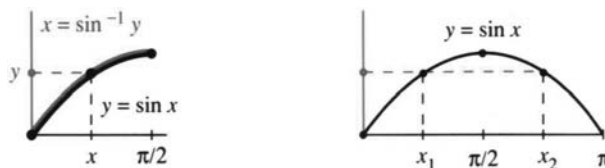
Fig. 4.5 Inverse exists (one x for each y ). No inverse function (two x 's for one y ).
