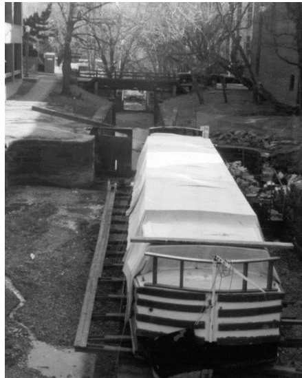
Figure 2 Remnants of the C&O Canal can still be seen in Georgetown in the District of Columbia. Note the long narrow shape of the boat, which is sized to squeeze into the locks, such as the one at the back of this picture.
