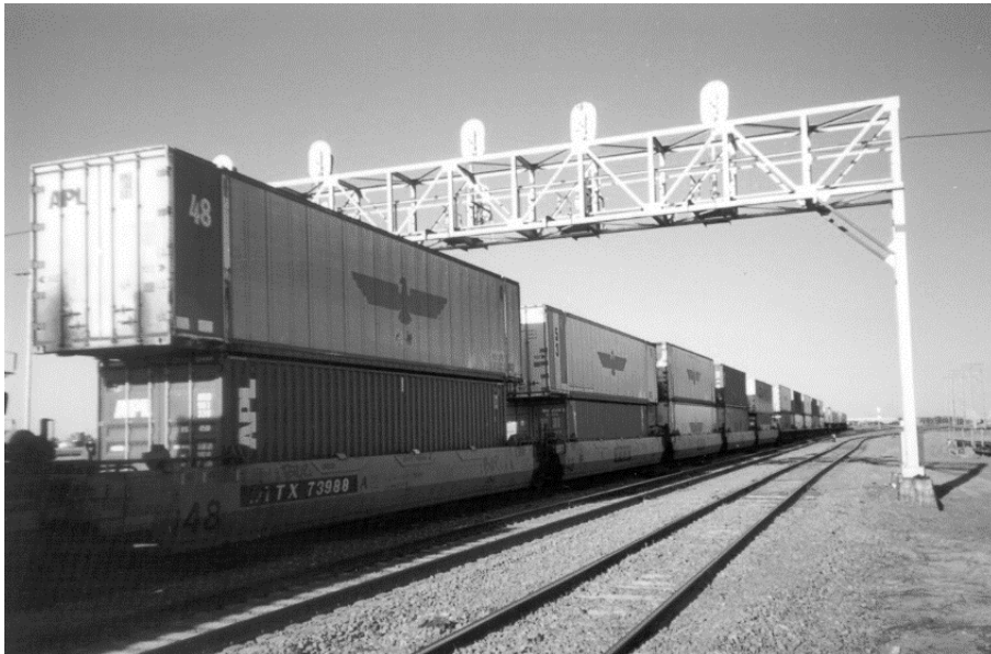
Figure 1 A double stack container train entering Union Pacific's Terminal in North Platte, Nebraska.
