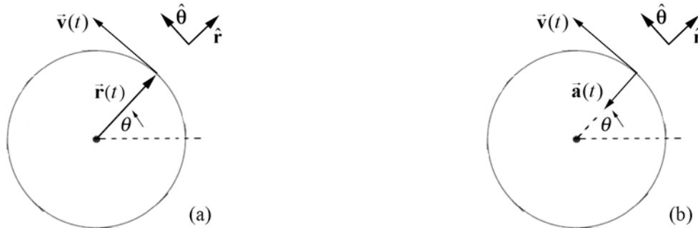
Figure 22.7 (a) Rotating position and velocity vector; (b) velocity and acceleration vector for uniform circular motion
