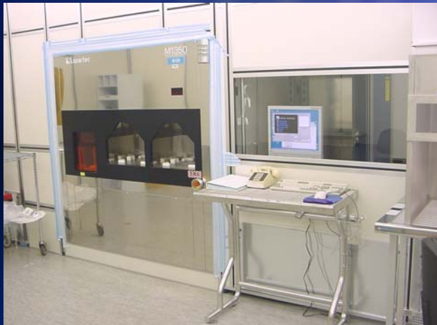
Commercial EUV blank inspection tool installed at Intel mask facility
