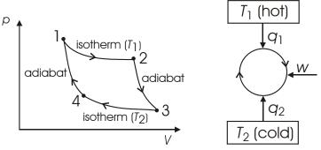
$\begin{array}{ll} 1 \rightarrow 2 & \text{isothermal expansion at } \mathcal{T}_1 \text{ (hot)} & \Delta U = q_1 + w_1 \\ 2 \rightarrow 3 & \text{adiabatic expansion } (q = 0) & \Delta U = w_1' \\ 3 \rightarrow 4 & \text{isothermal compression at } \mathcal{T}_2 \text{ (cold) } \Delta U = q_2 + w_2 \end{array}$
