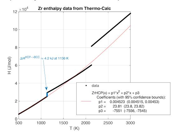
We determine the heat capacity model parameters from the polynomial coefficients, which Matlab lists as p1, p2, p3:
