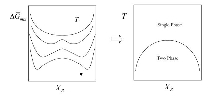
The boundary between the one- and two-phase regions which defines the miscibility gap is obtained by:
