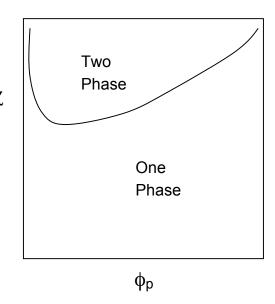
The critical concentration of polymer in a polymer-solvent mixture scales as  $N^{-1/2}$ . Note that the critical temperature (defined by  $\chi_{cr}$ ) is also fixed, in accordance with the phase rule.
