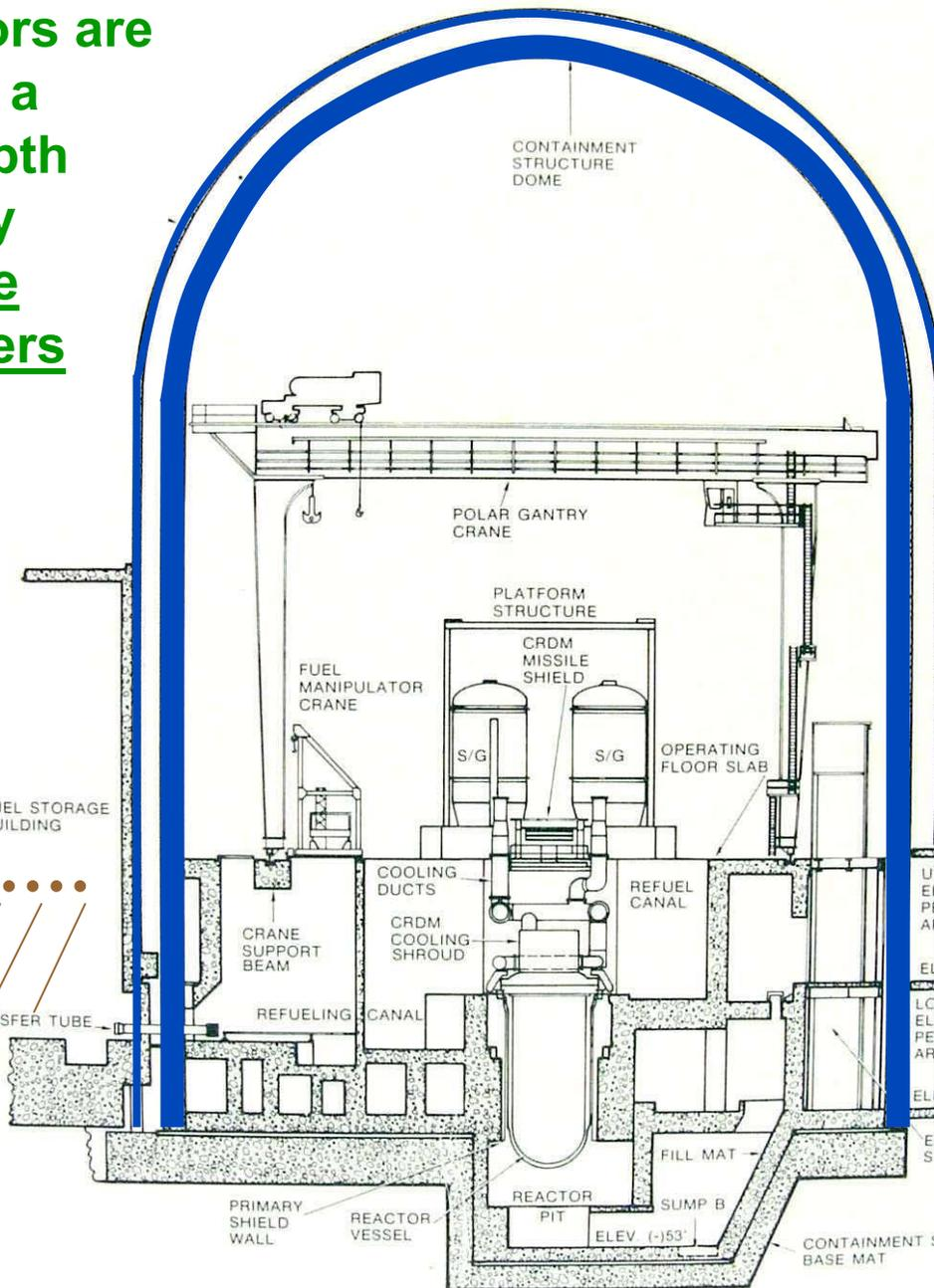
3) The containment building with double walls of thick steel-reinforced concrete:
