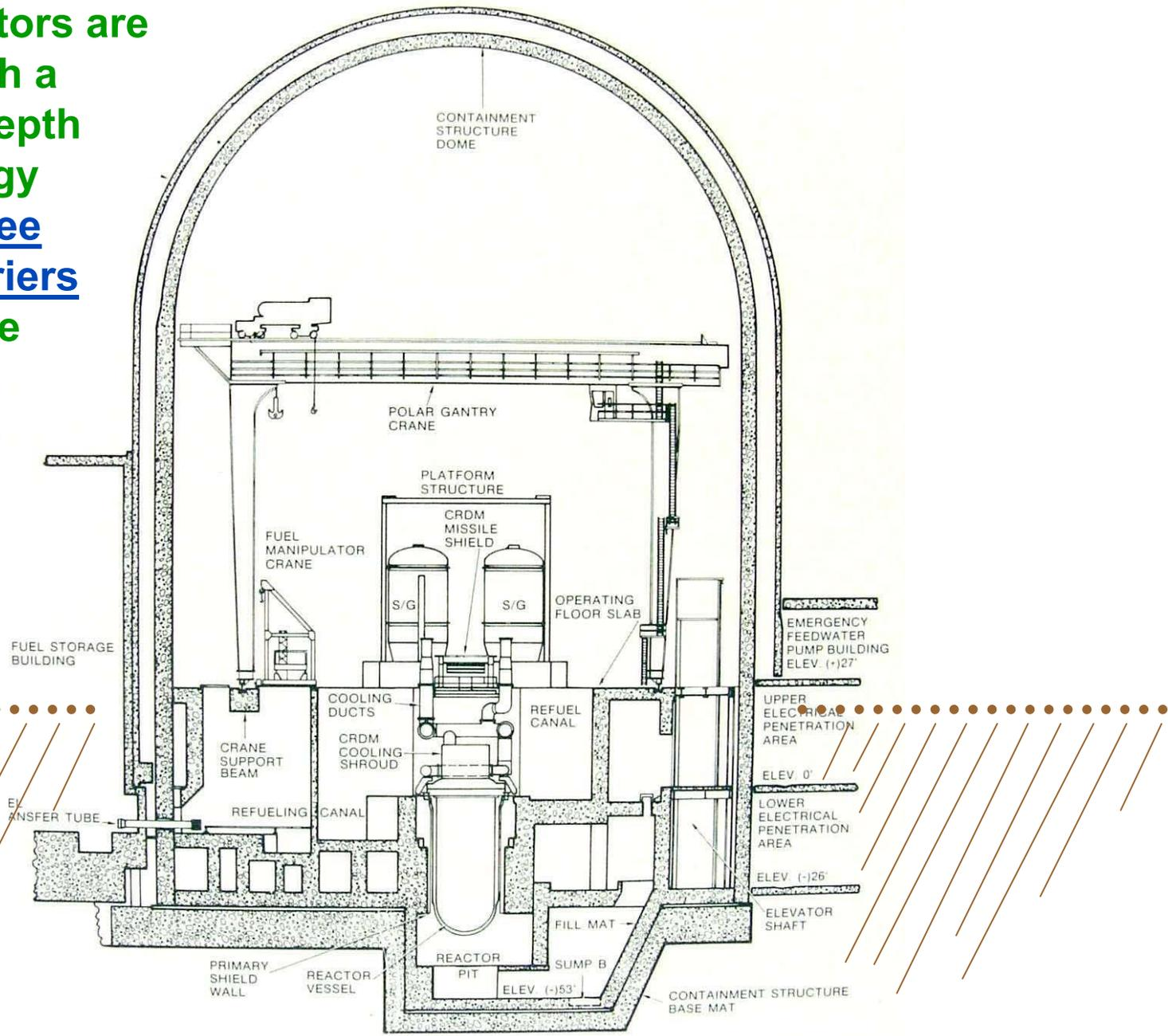
Nuclear reactors are designed with a defense-in-depth safety strategy that uses three physical barriers to prevent the release of radioactivity.
