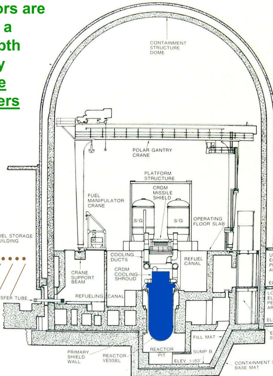
2) The reactor coolant system, including the reactor pressure vessel with walls of steel that range from nine inches to a foot
