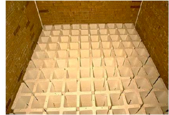
Figure 8: Firebrick regenerator for a glass furnace 19
