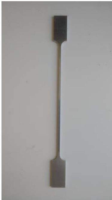
Figure 1: A Dogbone Specimen on which tensile testing will be performed
